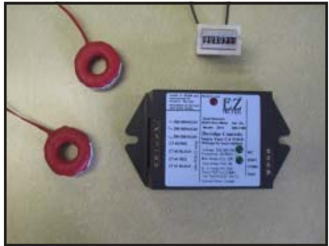
The Zion watt-hour meter
