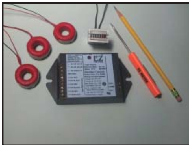
The Yellowstone watt-hour meter
