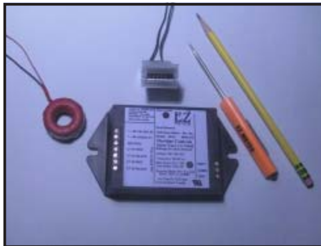
The Sequoia watt-hour meter
