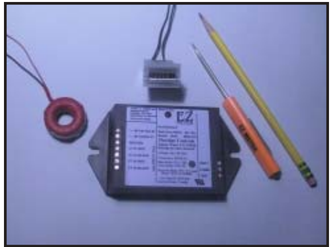
The Biscayne watt-hour meter
